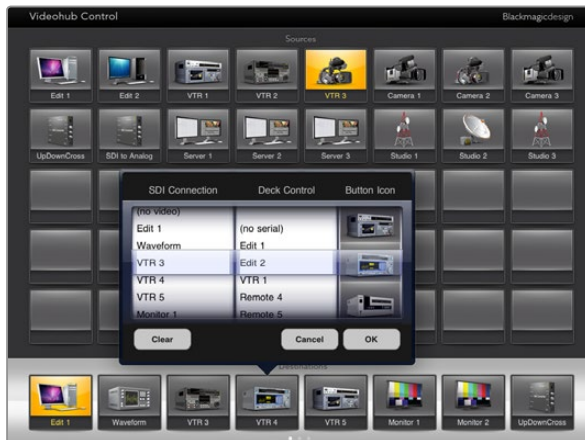
The Videohub Button Setup window allows you to set the SDI input or output connection, RS-422 deck control and the icon for the pushbutton.
